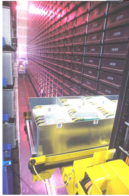
Automated Storage and Retrieval System, Defense Visual Information Center by Lance Cheung [Public domain], via Wikimedia Commons .
